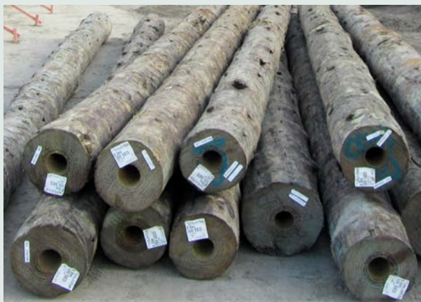
TTT Uglie MultiPoles have greater skin friction which is beneficial when used as foundation piles.
